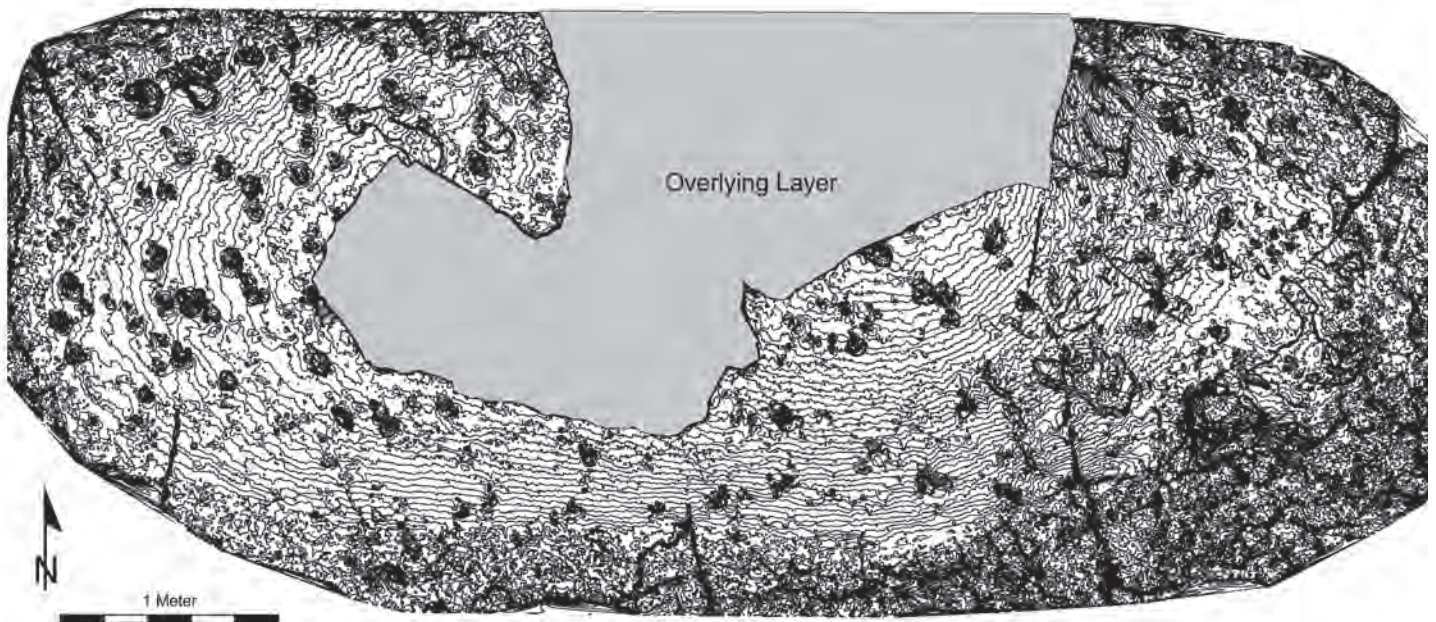
FIGURE 7. Topographic map of Tracksite UNLV-AZ-004, generated from photogrammetric data. Contour interval is 1 mm.
