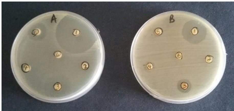
Figure of filter paper disk method experiment showing zones of inhibition, from Petersen, J. and S. McLaughlin. 2016. Laboratory Exercises in Microbiology: Discovering the Unseen World Through Hands-On Investigation. CUNY Academic Works. Accessed 2018.
